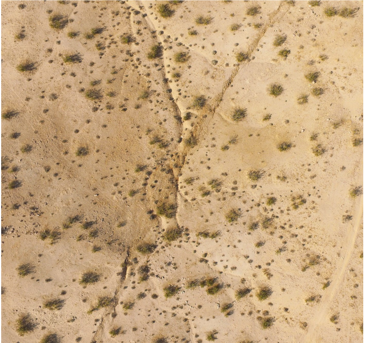
Figure 1-3F-1 UAS image of offset channels along the M6.4 rupture taken July 5, 2019.
