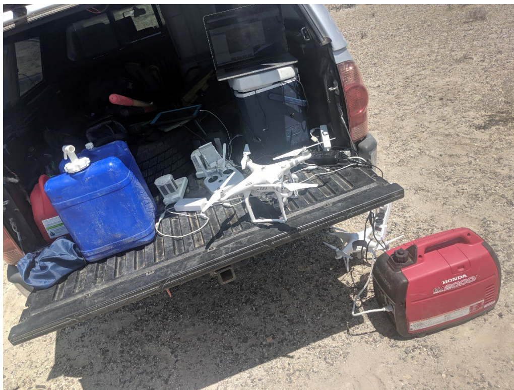
Running a generator to charge drone batteries in the field.
