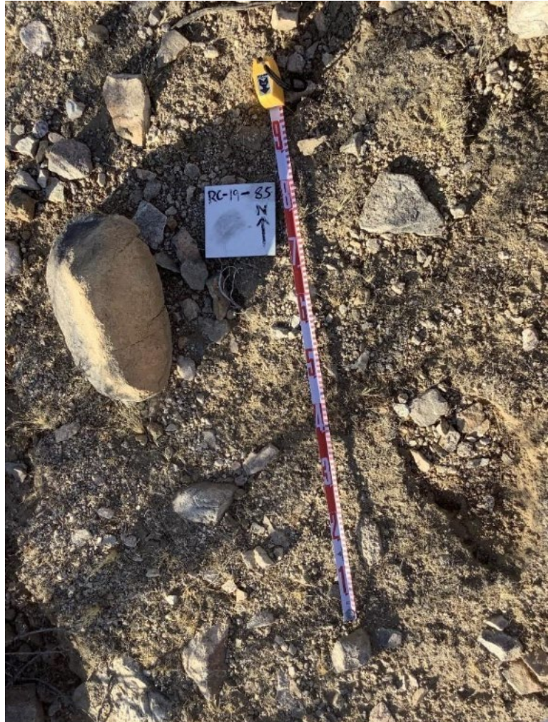
Figure 1-3C-2. Site set up, including clear view of clast and socket, whiteboard with site number and North arrow, and tape measure scale.
