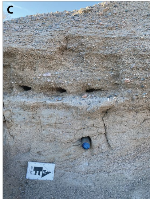
Figure 1-1c-6. (A) Simplified stratigraphic column and unit descriptions of the 607 m beach ridge site (South exposure). White star indicates location of luminescence sample (see Table 1-1c-1). Photographs of: (B) bluff exposure of alluvial and shoreline deposits; and (C) luminescence sample location of SL015 in sandy foreset overlain by stratified sandy gravel backsets and topsets.
