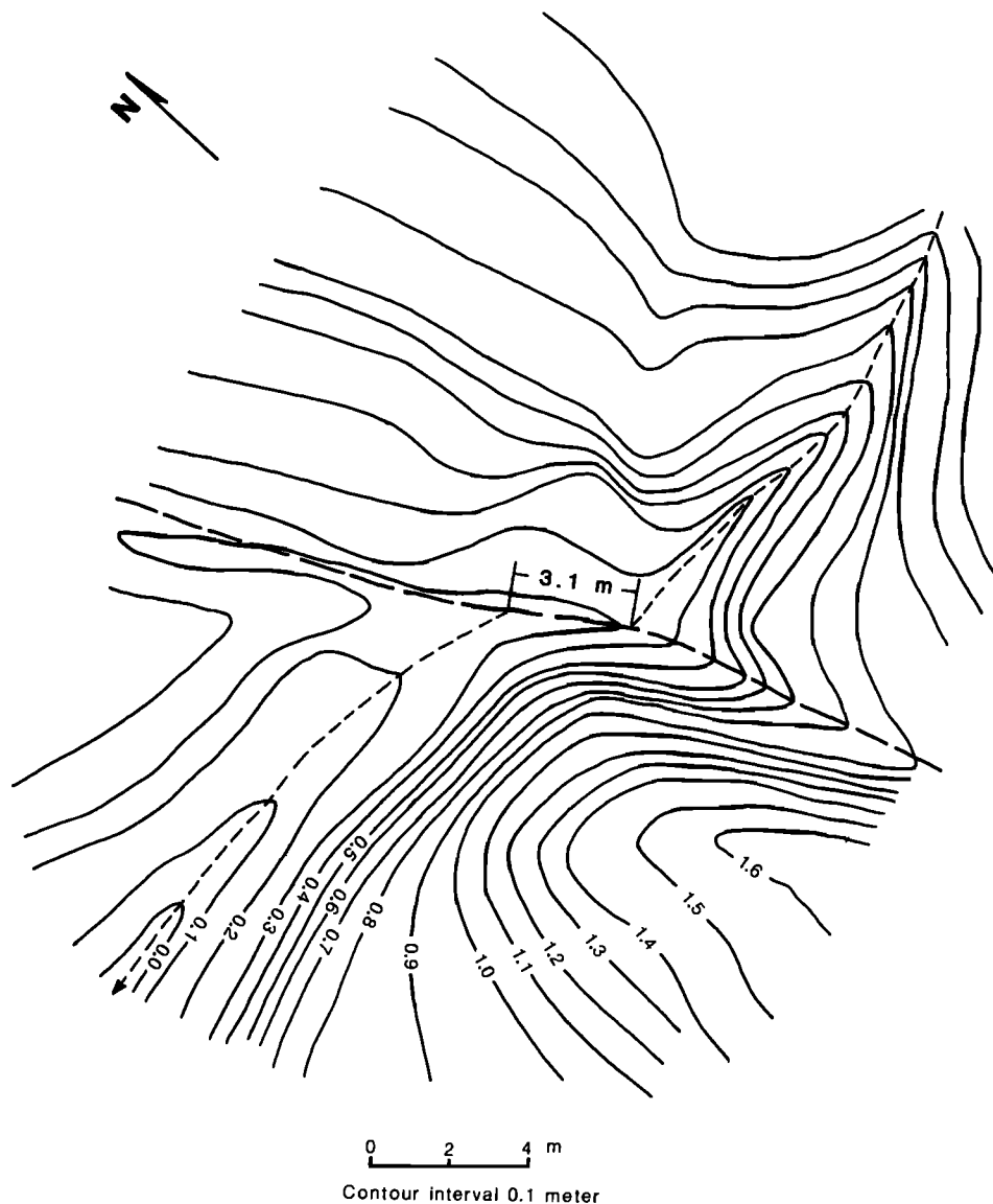
Fig. 7. Topographic contour map of offset stream near Manly Peak Canyon (Site 4). Thick lines represent fault scarps. Dashed line represent the central line of the stream channel. The right-lateral displacement is 3.1 \pm 0.4 m by matching up central lines between upstream and downstream channels. The elevation is arbitrary.
