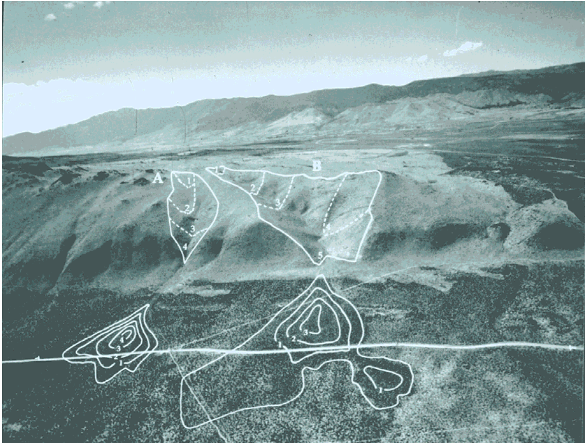
Fig. 4-2. Taken from Granger et al., 1996. Oblique aerial photo of the Fort Sage Mountains fault scarp, showing catchment boundaries (solid lines), subcatchment boundaries (dotted lines) and alluvial fan thickness contours (in m, from depths to beach sands below). The fans have accumulated each catchment's erosional debris since Lake Lahontan retreated from the scarp base ~16 ky ago. Thus the fans record long-term erosion rates of the contributing areas.
